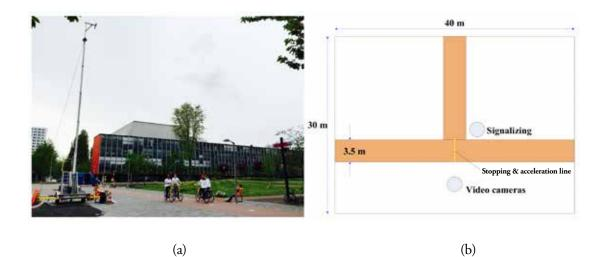
Figure 1: Overview of monitoring setup at the TU Delft campus: (a) a snapshot taken during the experiment; (b) a schematized aerial view of the experimental area monitored by two cameras
