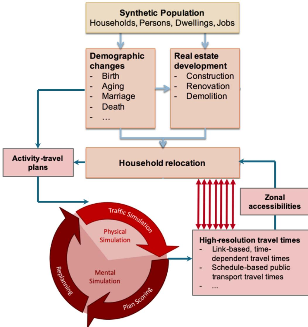
**Figure 1:** Schematic visualization of FABILUT model. Blue arrows denote information whose generation is finished before it is made available to another module. Red arrows denote individualized queries from a module to another component. The requested information is unknown before the requesting module is active.
